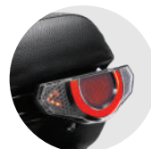
Rear brake light with integrated turn indicator
